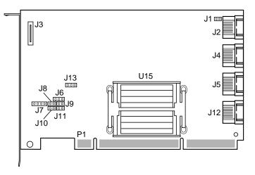
Verify that the jumper settings on the MegaRAID SATA 300-8X are correct. The jumpers are set at the factory, and you probably do not need to change them. The following table describes the jumpers and connectors on the RAID controller.
