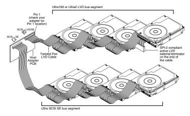
Figure 3. Cable connections and external termination
