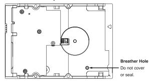
**Caution.** Do not cover, seal, or insert any object into this hole. This hole has two purposes:
