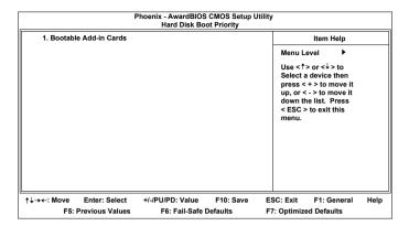
This is for setting the priority of the hard disk boot order when the "Hard Disk" option is selected in the "[First/Second/Third] Boot Device" menu item.
