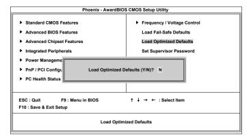
This option is for restoring all the default optimized BIOS settings. The default optimized values are set by the mainboard manufacturer to provide a stable system with optimized performance.
