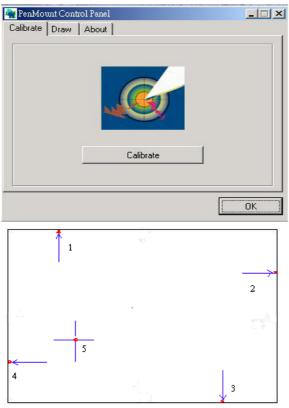
• Draw Test or demonstrate PenMount touch screen operation, also the touch location is shown on the display, touch "DRAW" to start.
