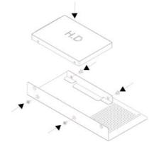
2. Install the HDD module onto main chassis.
