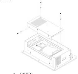
2. Remove the HDD from rear cover.
