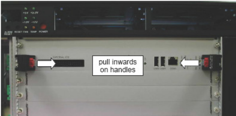
Figure 2-2: Latching the cPCI module handles securely.
