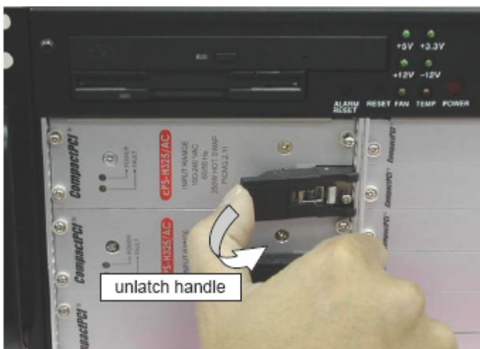
Figure 2-3: Unlatch the PSU module handle
