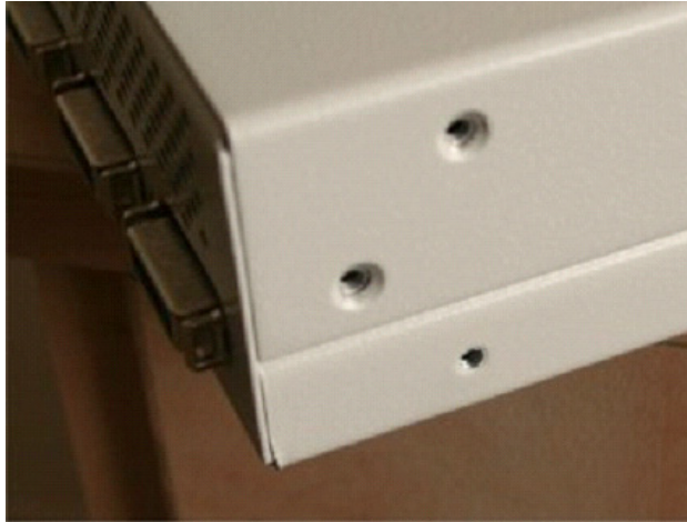
Figure 4: Rear Panel Side with Ear Screws Removed
