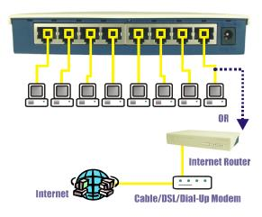
Any EZ800-S port can be used as an uplink port because the EZ800-S will auto-detect uplink.
