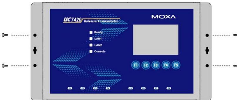
**Figure b. UC-7400 Series Universal Communicator—Wall Mounting Brackets (top view)**
