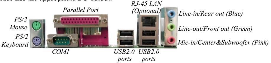
Figure 3: I/O ports
