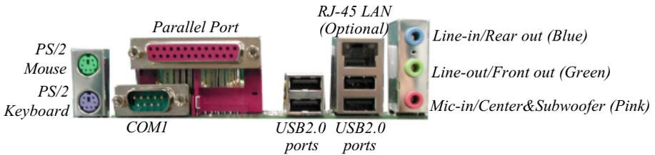
Figure 11 - I/O Ports
